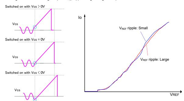
Figure 19 Changes in on-time determined by switching-on timing in the [B] region
