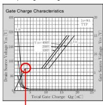
Qg (Vth): Accumulated charge until the voltage reaches the gate threshold
