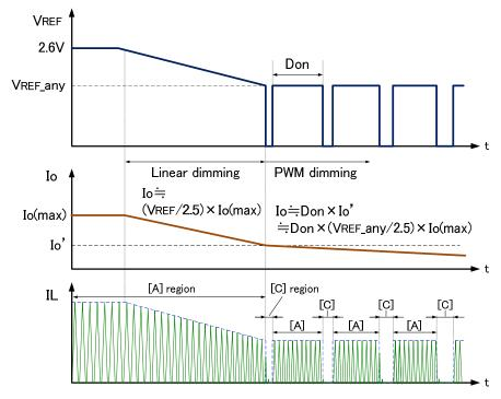
Figure 23 Combination of linear dimming and PWM dimming
