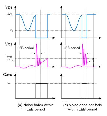
Figure 18 Example of false detection due to switching-on noise
