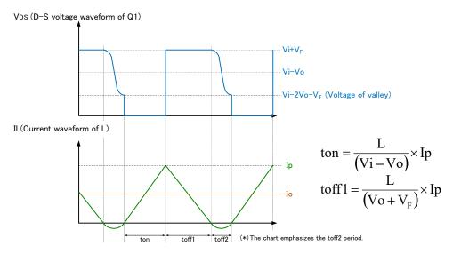
Figure 5 Basic operation waveforms
