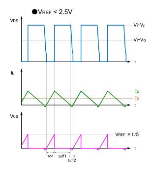
Figure 15 Operation waveforms in [A] frequency modulation region
