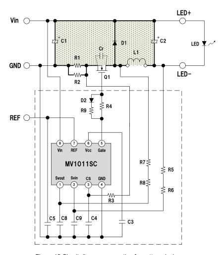
Figure 12 Circuit diagram accounting for pattern design
