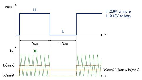
Figure 22 Example of PWM dimming operation
