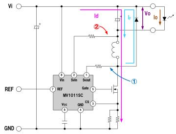
Figure 1 CRM step-down chopper circuit
