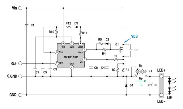
Figure 11 Circuit configuration of High-side drive
