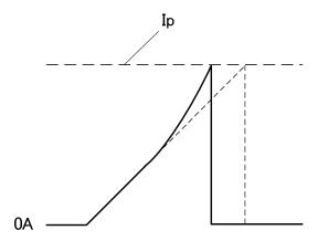
Figure 6(b) MOSFET current waveform at inductance drop
