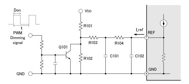
Figure 24 Example of PWM dimming signal smoothing circuit
