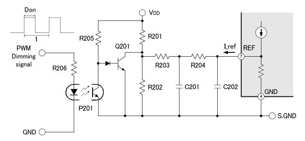
Figure 25 Example of dimming circuit in high-side drive configuration
