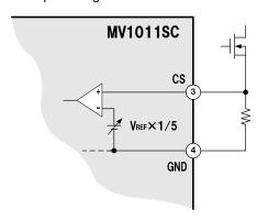
Figure 14 CS pin internal circuit diagram
