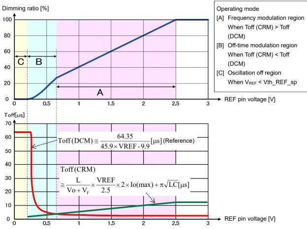
Figure 13 Relationship of REF pin voltage V<sub>REF</sub> to dimming ratio and to off-time Toff
