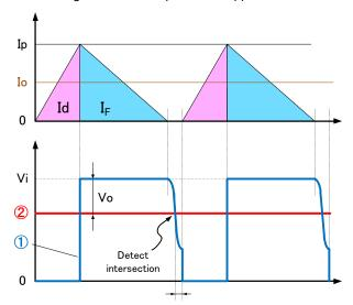
Delay in detection by IC + gate delay
