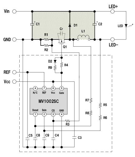
Figure 11 Circuit diagram accounting for pattern design
