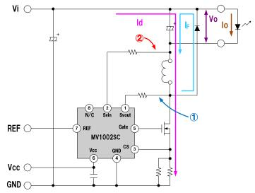
Figure 1 CRM step-down chopper circuit
