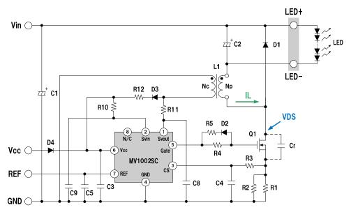
Figure 9 Configuration of a winding voltage supply
