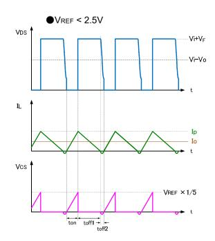
Figure 14 Operation waveforms in [A] frequency modulation region
