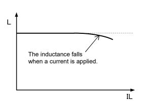
Figure 6(a) Inductor's DC bias characteristics
