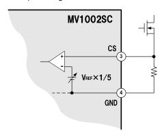
Figure 13 CS pin internal circuit diagram
