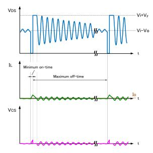
Figure 20 Operation waveform in the [C] minimum dimming region
