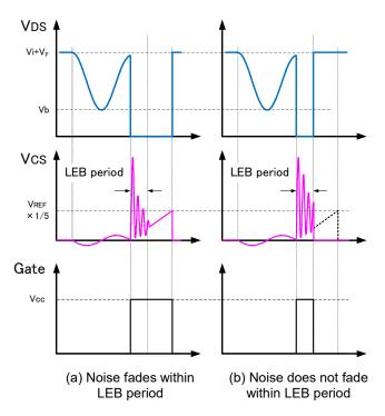
Figure 17 Example of false detection due to switching-on noise
