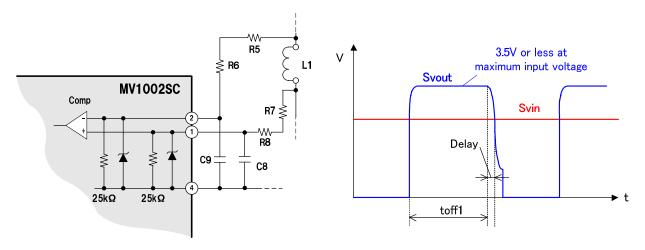
Figure 7 Zero current detecting operation waveforms and internal circuit diagram
