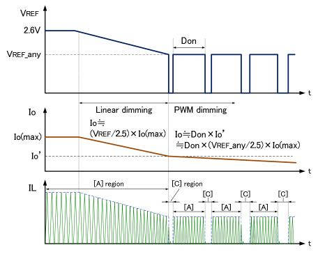
Figure 22 Combination of linear dimming and PWM dimming
