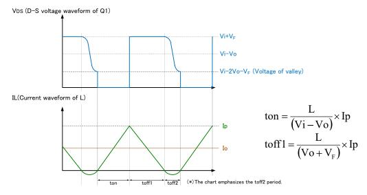
Figure 5 Basic operation waveforms
