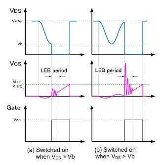
Figure 16 Example of switching-on noise caused by V<sub>DS</sub>
