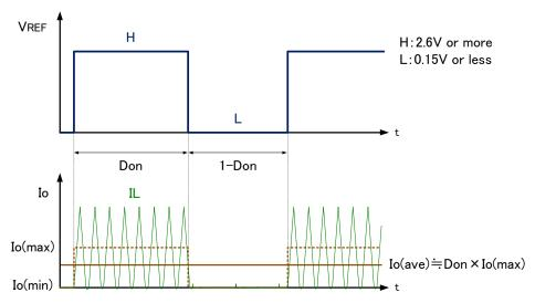
Figure 21 Example of PWM dimming operation
