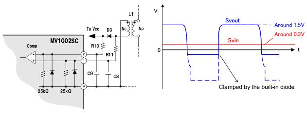
Figure 10 Waveforms of Svin and Svout pins when an auxiliary winding is used
