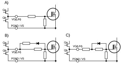
Fig. 3 . Gate drive circuits
