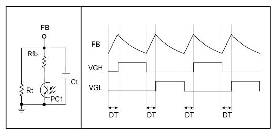
Fig.4 . FBL – VGL/VGH timing
