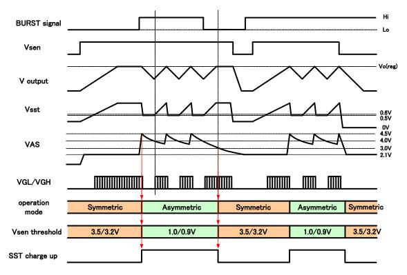
Fig. 17 Burst mode operation timing
