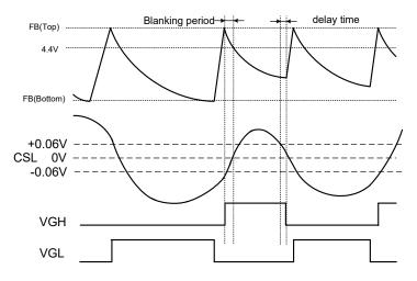
Fig. 10 . Anti-capacitive mode protection timing
