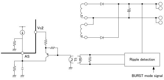
Fig. 18 BURST w/external signal configuration example
