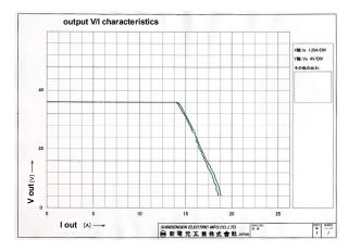
Fig. 21 OLP characteristics example
