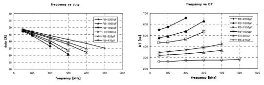
Fig. 5. Gate output duty/dead time vs frequency
