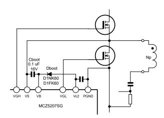
Fig. 14 Boot Strapping circuit
