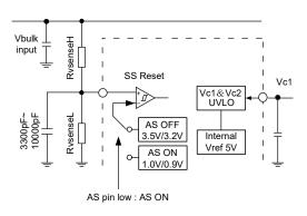
Fig.26 Vsen internal circuit
