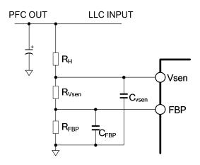
Value of  $R_{\text{FBP}}$  is obtained from formula (20). Value of  $R_{\text{Vsen}}$  is obtained from formula (21).
