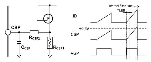
Fig.10 CSP circuit example and timing diagram
