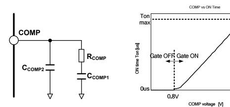
Fig.7 Example circuit connected with COMP
