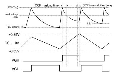
Fig.16 Over current protection
