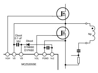
Fig.20 Boot Strapping configuration
