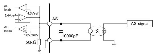
Fig.21 AS mode circuit example
