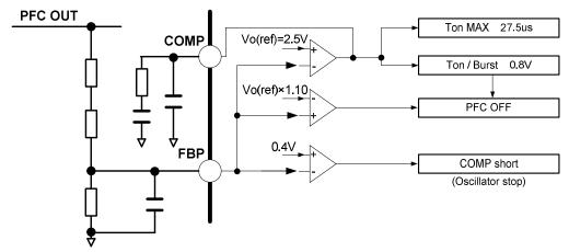
Fig.6 PFC gate drive circuit
