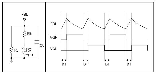
Fig.12 FBL timing diagram
