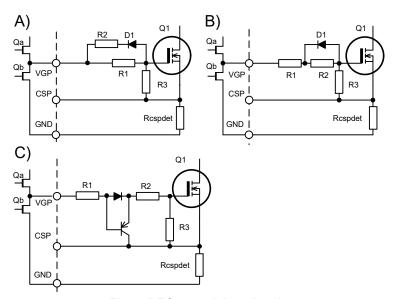
Fig.5 PFC gate drive circuit
