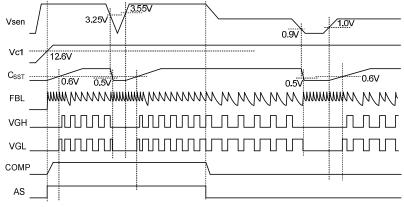
Fig.14 Vsen output timing diagram
