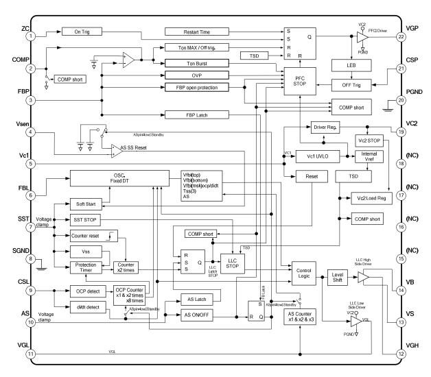
Fig.1 MCZ5205SE internal block diagram
