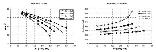
Fig.13 Duty/dead time vs frequency
