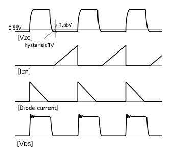
Fig.9 PFC block timing diagram (ZC)
