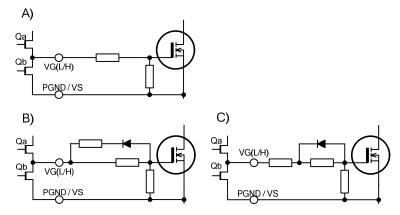
Fig.11 LLC Gate drive circuits
