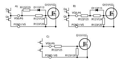
Fig.20. Gate driving configuration
