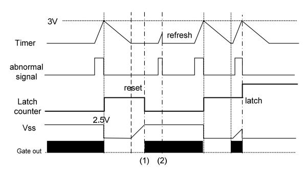
Fig.18. Timer delayed burst and latching timing chart
