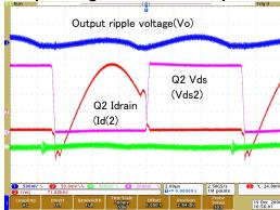
Fig.3 Vds / Idrain / Vo ripple
