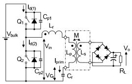
Fig.2 simplified dc/dc converter
