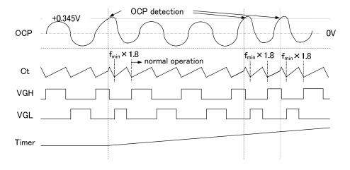
Fig.14. OCP Timing diagram
