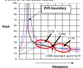
Voltage vs.frequency characteristics are shown in Fig.5. LLC converter operates in above-resonance region. (above ZVS boundary)
