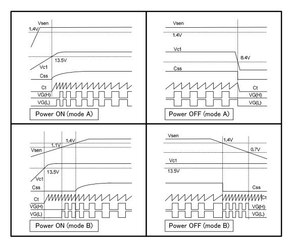
Fig 6. Power ON / OFF timing diagram
