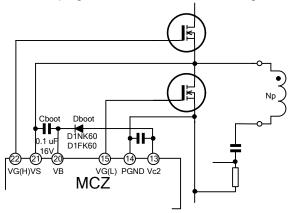
Fig.19. Boot Strapping configuration
