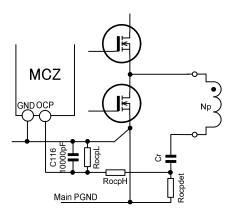
Fig.15. Main resonant current detecting configuration
