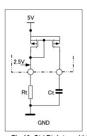
Fig.10 Ct / Rt internal block
