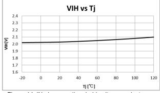
Figure 14 IN pin upper threshold voltage against junction temperature
