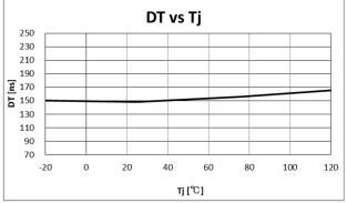
Figure 24 Fixed dead time against junction temperature
