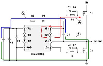
Figure33 Bootstrap circuit basic operation
