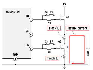
Figure 38 Track inductance and reflux current schematic
