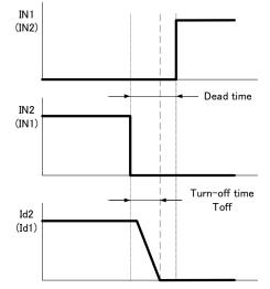
Figure 34 Relationship between dead time and turn-off time
