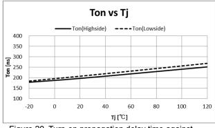
Figure 20 Turn-on propagation delay time against junction temperature
