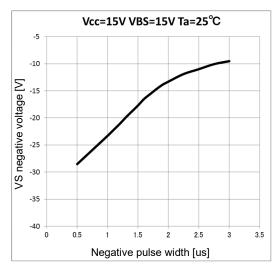
Figure 37 VS pin negative voltage tolerance (typical data)
