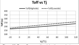
Figure 22 Turn-off propagation delay time against junction temperature
