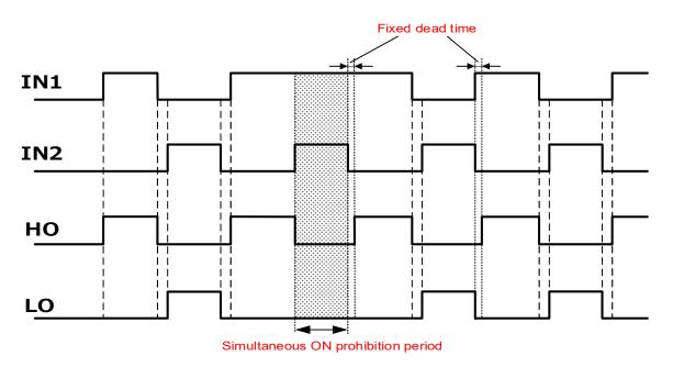
Figure 32 Simultaneous ON prevention timing chart
