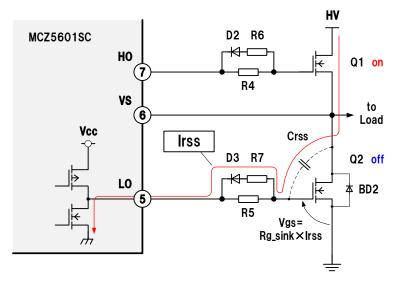
Figure 36 Self turn-on operation (Irss current path)
