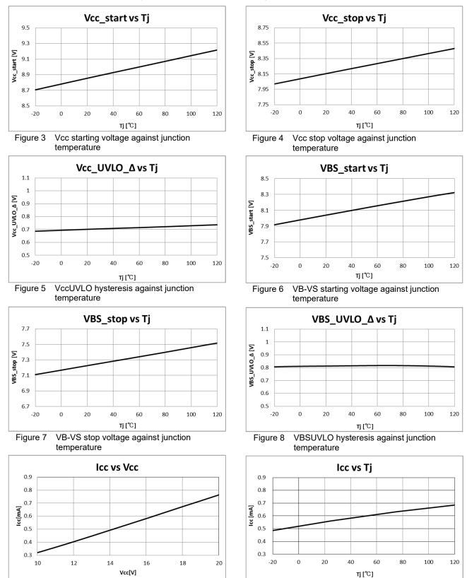
Figure 9 Vcc consumption current against Vcc pin applied voltage
