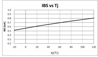
Figure 12 VBS consumption current against junction temperature
