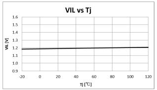
Figure 16 IN pin lower threshold voltage against junction temperature
