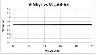
Figure 17 IN pin threshold hysteresis voltage against power supply voltage
