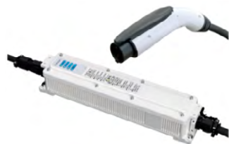
Model: PM-CS09-M-CG Output: 6kW (200V/30A) Installation: Ground, wall surface, ceiling, diagonal surfaces, unseen places, etc. Functions: Wireless control/output current adjustment
